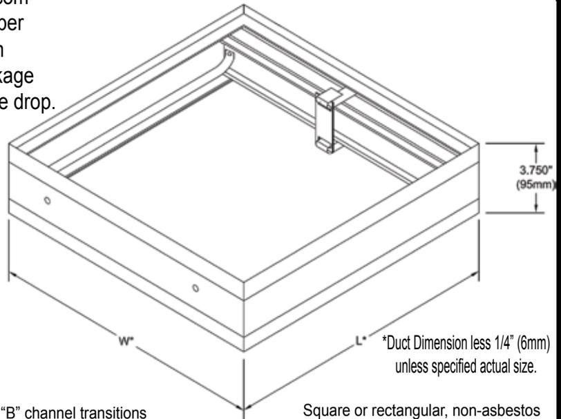
Designed and tested in accordance to standards: UL 555C, ULC S112.2. Labeled and listed by UL/ULC under File #R27747. They meet all the NFPA-90A, IBC Code, and other major code requirements for Ceiling (Radiation) Dampers.
